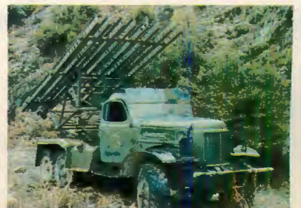
Afraid to commit first-line equipment in war they may not win, Soviets deploy WWII-vintage 132mm BM-13-16 artillery rockets on antiquated ZIL-151 trucks.
