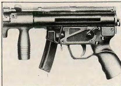
**Heckler & Koch MP5K submachine gun is designed for clandestine operations. Note single open notch rear sight on this particular variant, vertical foregrip and absence of buttstock.**
