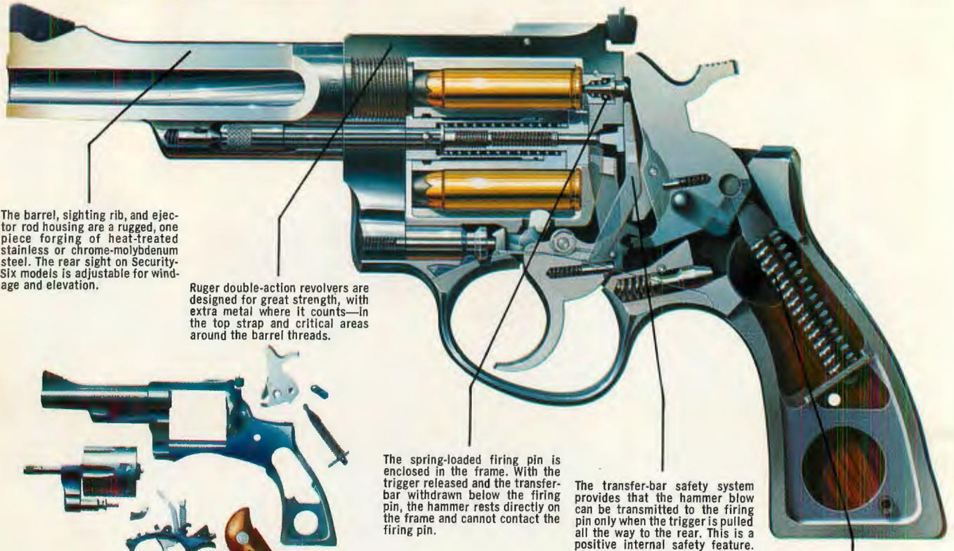
The barrel, sighting rib, and ejector rod housing are a rugged, one piece forging of heat-treated stainless or chrome-molybdenum steel. The rear sight on Security-Six models is adjustable for windage and elevation.
