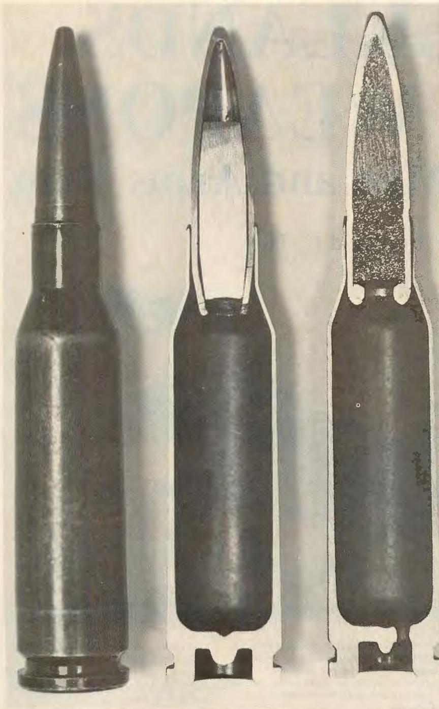
Cut examples of two different types of Soviet 5.45x39mm ammo issued — and captured — in Afghanistan: one two-part solid core, the other single, symmetrical lead core leaving hollow under steel nose.
