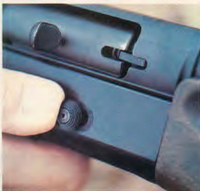
Newly-designed and installed push-button cartridge-release overcomes only military/police objection to Model 121.
