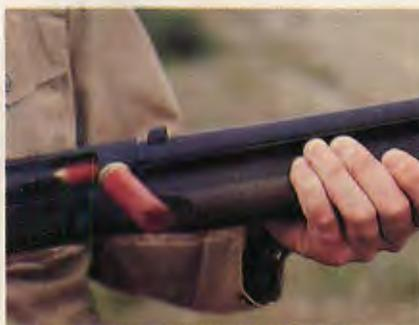
Other guns of this type have utilized short recoil. Ammunition-sensitive, but fairly reliable, recoil-operated shotguns are noted for whaling the hell out of the shooter. Felt recoil is severe and they have given way to gas-operated shotguns.
