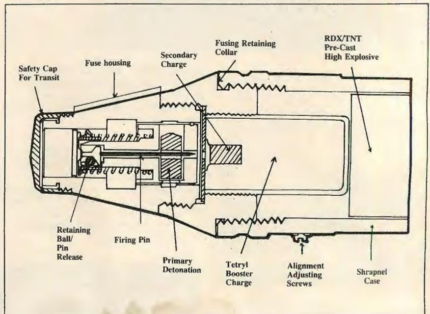
Cutaway diagram showing OG-7 components.
