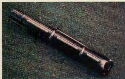
Stamped sheet-metal receiver cover ribbed for structural support as with the AKM.
