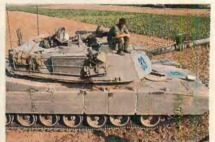
ABOVE: M1 Abrams MBT, equipped with commander's M2 HB Cal. .50 machine gun, has 105mm M68 E1 main gun. U.S. will update gun to German Rheinmetall 120mm in 1984.
