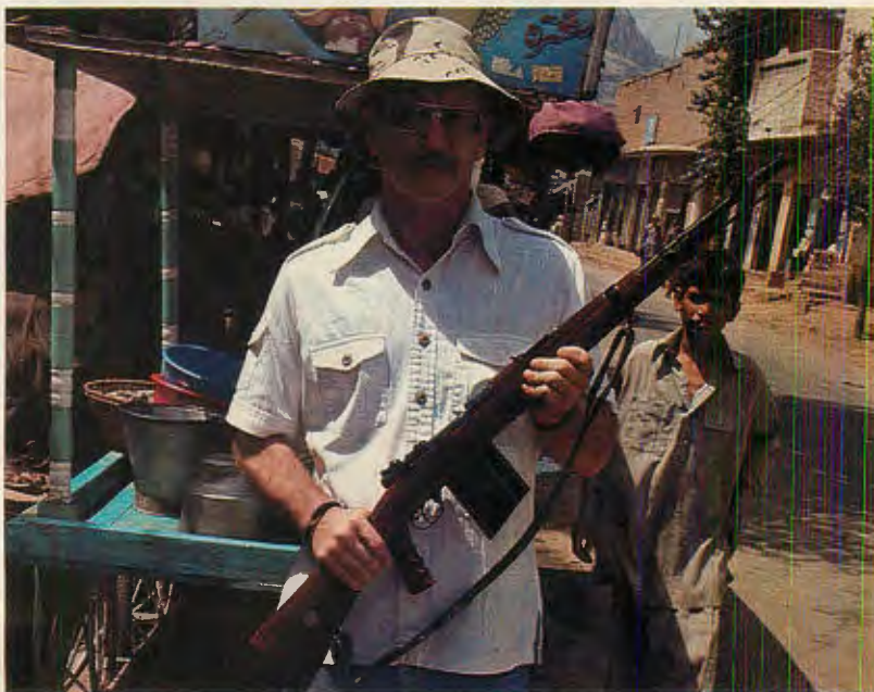
Gunsmithing limited only by imagination: SOF Editor/Publisher Robert K. Brown holds shop-made custom rifle that exactly copies "Iranian" Mausers, except for short barrel, flash suppressor, 7.62mm NATO chamber, FN 20-round box magazine, and M14A1-style pistol-grip.
