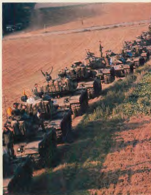
ABOVE: M1 Abrams MBT, equipped with commander's M2 HB Cal. .50 machine gun, has 105mm M68 E1 main gun. U.S. will update gun to German Rheinmetall 120mm in 1984.
