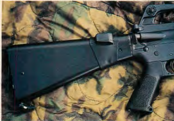
RIGHT: M16A1 battle rifle fitted with Arm-Tec's Fire Control Gun Stock. Hinged projections provide positive platform for shooter's cheek, stabilizing sight picture. CENTER AND BELOW: Arm-Tec's Fire Control Gun Stock with special adaptor for installation on Heckler & Koch 91.
