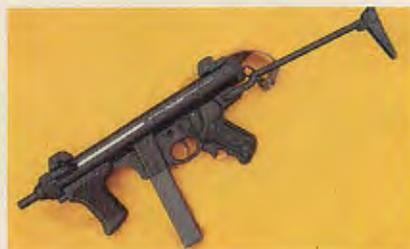
ABOVE: Field-stripped Beretta Model 12S. Disassembly can be done in matter of seconds by removing barrel butt and end cap. LEFT: Beretta Model 12S with stock extended. First produced in 1959, Domenico Salza's design is compact, lightweight and accurate.
