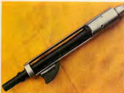
ABOVE: Telescoping bolt and barrel from Beretta Model 12S. Of total barrel length of 7.9 inches, 5.9 inches lie inside bolt-block at moment of firing, reducing muzzle climb to absolute minimum. BELOW: Trigger assembly on Beretta Model 12S shows fire-selector switch for Rapid, 1 (semiauto) and Safe.
