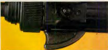
ABOVE: Model 12S barrel nut and post-type front sight from above. Note large ears protecting sight. Cast-steel retracting handle is on left of barrel. BELOW: Model 12S rear sight, end cap latch and end cap. If end cap is not completely tightened, latch remains raised.
