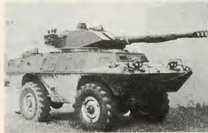
Cadillac Gage V-150 armed with turret-mounted Belgian Cockerill MK III 90mm gun. In its squad carrier variation, the V-150 is supposed to carry nine men. Photo: Edwin W. Besch
