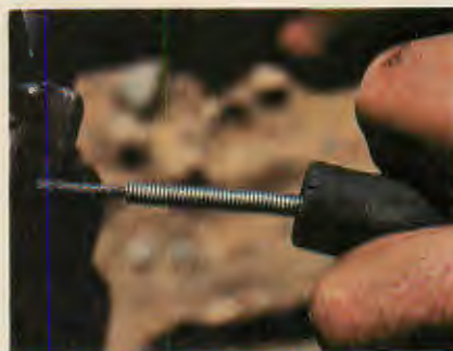
RIGHT: Running straight out the rear of the receiver, cocking handle cable is fixed to back of the block.
