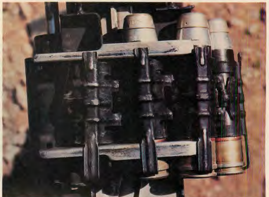
BELOW: Proper AGS-17 loading procedure: curved, parallel prongs on top of sheet-metal feed block are inserted between cartridges and links.
