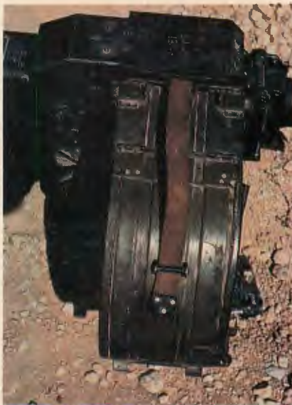
BELOW: Proper AGS-17 loading procedure: curved, parallel prongs on top of sheet-metal feed block are inserted between cartridges and links.
