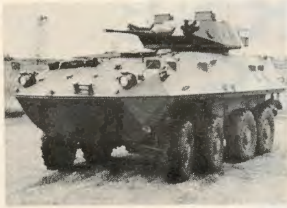
Swiss MOWAG (Motorwagenfabrik) Piranha 8x8, armed with M242 25mm chain gun, is one of two foreign USMC LAV candidates. Photo: USMC
