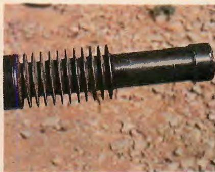
ABOVE: Closeup of cooling fins.
