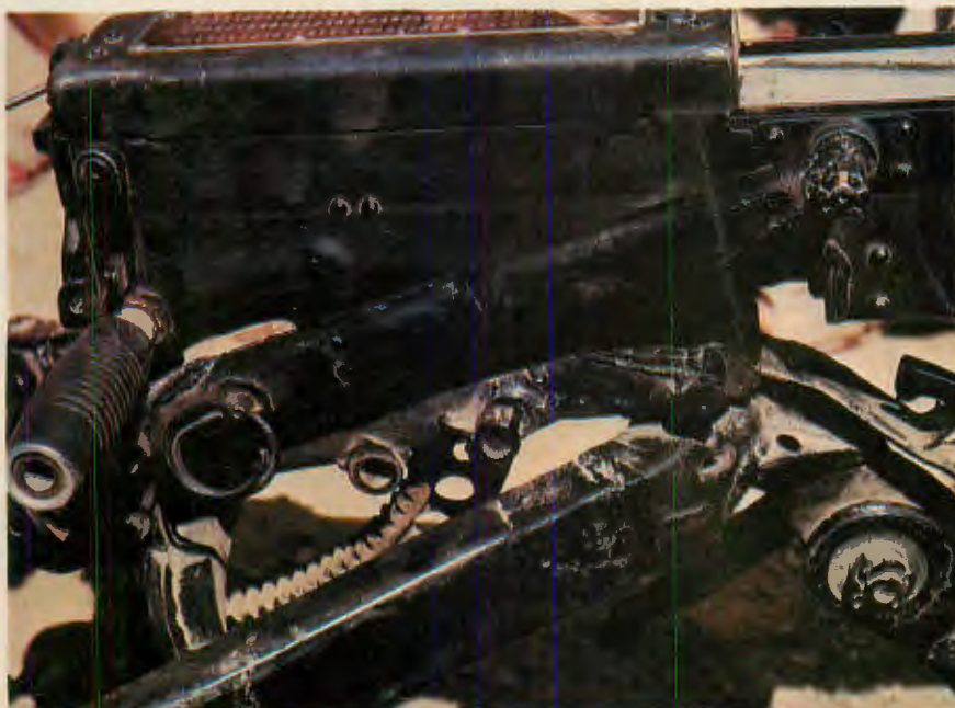
RIGHT: Running straight out the rear of the receiver, cocking handle cable is fixed to back of the block.
