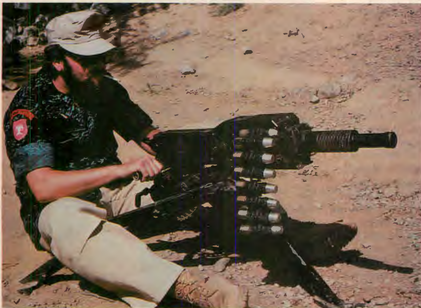
ABOVE: Blowback operation, heavy bolt and light tripod gave high recoil and low control, so Coyne impersonates sandbag by sitting on rear tripod legs for firing session. Villagers not visible, since they hid behind rock berm, thinking launcher unreliable.
