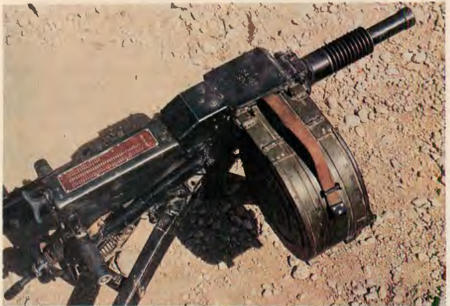
BELOW: Proper AGS-17 loading procedure: curved, parallel prongs on top of sheet-metal feed block are inserted between cartridges and links.
