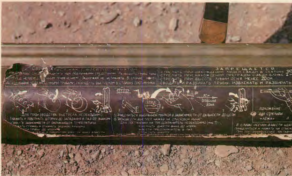
ABOVE: Cyrillic directions in Russian for RPG-18 are supplemented by pictures to facilitate use by often illiterate and non-Russian-speaking Oriental and Turkic Soviet Army conscripts. LEFT: Inside and out, virtually a dead ringer for U.S.-issue LAW. RPG-18 differs little except for longer missile, shaped-charge warhead and directions in Russian. Photos: Peter G. Kokalis
