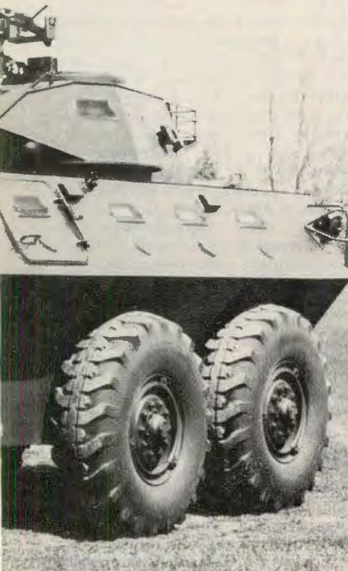
ABOVE: Cadillac Gage V-300 6x6 is one of four Marine Corps light assault (squad carrier) candidates. Vehicle is armed with M242 25mm chain gun. Photo: USMC
