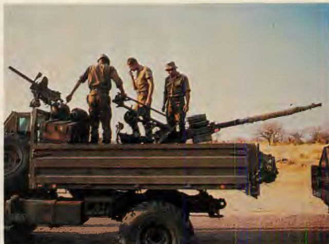
ABOVE: South African Army truck becomes makeshift weapons platform with forward-mounted Browning .30-caliber 1919A4 machine gun, and Oerlikon 20mm belt-fed cannon KAA (formerly designated 204 GK) in rear. Truck is part of convoy heading north into captured SWAPO territory in southern Angola.
