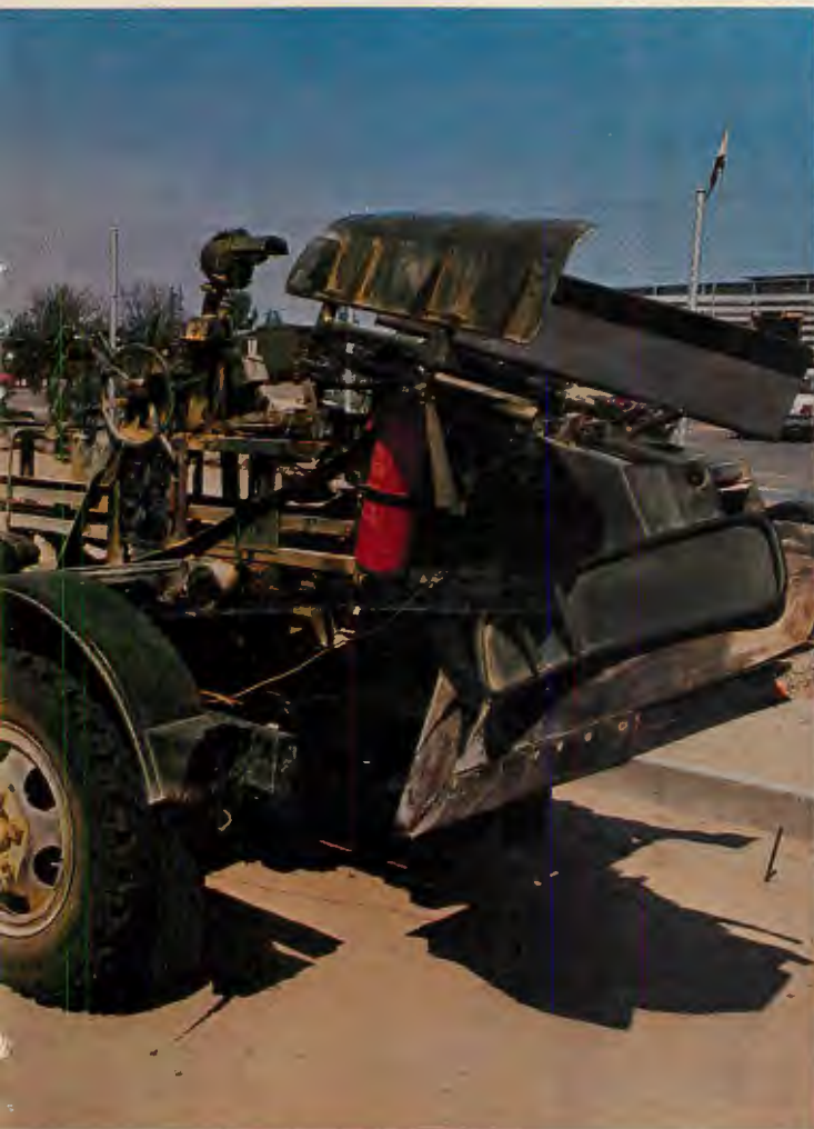
ABOVE: South African Army truck becomes makeshift weapons platform with forward-mounted Browning .30-caliber 1919A4 machine gun, and Oerlikon 20mm belt-fed cannon KAA (formerly designated 204 GK) in rear. Truck is part of convoy heading north into captured SWAPO territory in southern Angola.
