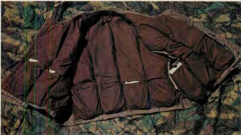
CENTER LEFT: Inner liner of Soviet flak-jacket. Elongated pockets hold single heat-sealed plastic packets stuffed with partially processed cotton wadding.
