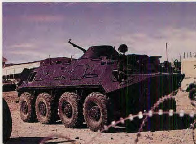
ABOVE: Amphibious, wheeled Russian APC designated BTR-60PB brandishes coaxial-mount 7.62mm PKT and heavy 14.5 KPV machine guns. LEFT: Tanker sleeps on Russian T-72, latest Warsaw Pact main battle tank. LOWER LEFT: APC crewman checks and performs light maintenance on M113 after tank "battle." LOWER RIGHT: Between battles "Red" tank crewmen pose next to T-72. Wearing replica Russian tanker berets, crewmen perform routine field maintenance.
