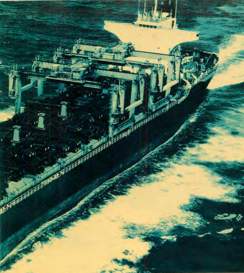
Saving space by separate shipment, SS Pittsburgh carries wheeled chassis for hauling containers by tractor/trailer. Photo: Skyfotos
