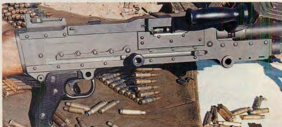
Closeup of FN MAG general-purpose machine-gun receiver. Failure occurred in front four cross bolts as discussed in text. Photo: Peter G. Kokalis
