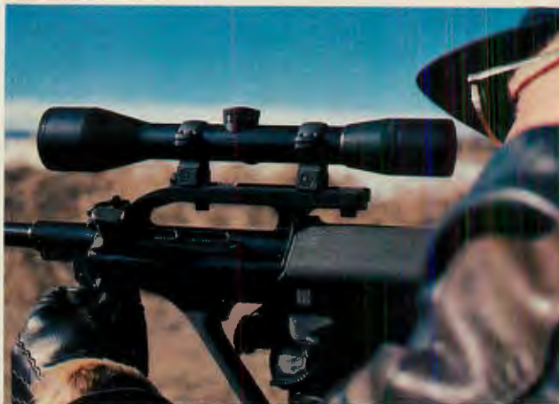
Robert K. Brown fires AUG Heavy Barrel Automatic Rifle with 24-inch barrel and 6x Kahles scope.
