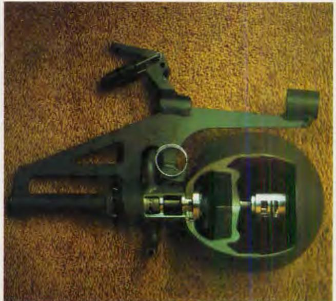
Cutaway RAW shows arming mechanism, payload and blast-directing aluminum shell.
