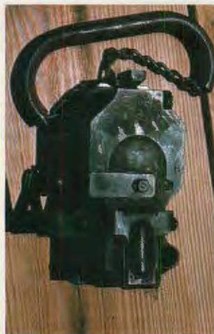
**ABOVE:** Outside of M85 backplate group with solenoid plunger and trigger.
