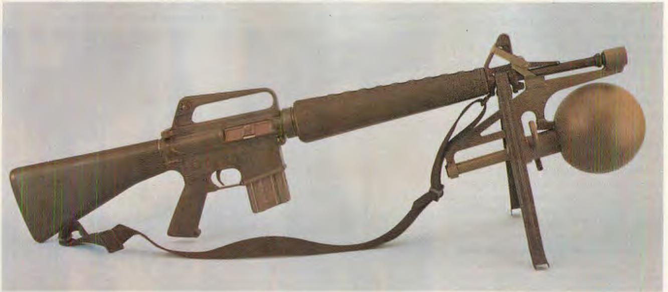
Six-pound RAW turns AR-15 into blockbuster. Armor- and masonry-penetrating rocket-propelled projectile has frag, smoke, gas and Willy Peter variants.
