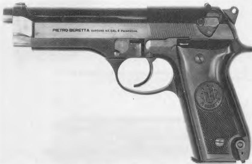
Original Beretta entry as U.S. service sidearm, M92S had rotating firing-pin safety but Army barred butt mag-release button. Photo: Beretta
