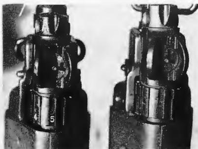
**FN FAL (right) conveniently marked on gas plug, front sight, and gas-regulator sleeve; marks economically but inconveniently missing from FN LAR.**
