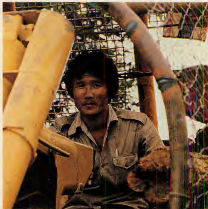
TOP: D-6 Caterpillar tractors with logs bolted to driver’s cage for protection from small-arms fire have cut deep into previously CPT-controlled areas. Road construction and security units faced problems of jungle and enemy with overwhelming courage and conviction. ABOVE: One of many civilian drivers who have made this hazardous project a success. Wire mesh and logs are bolted and wired to driver’s cage of D-9 Caterpillar tractor. Mines and 57mm recoilless-rifle fire were most discouraging weapons used by CPT.
