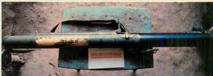
TOP: New Soviet RPG-18 (RPG-76) in the collapsed carrier position. Note firing diagrams using easy-to-understand drawings on sideplate. Similar in construction to U.S. LAW, MAW and HAW weapons (Light, Medium and Heavy Anti-tank Weapons).
