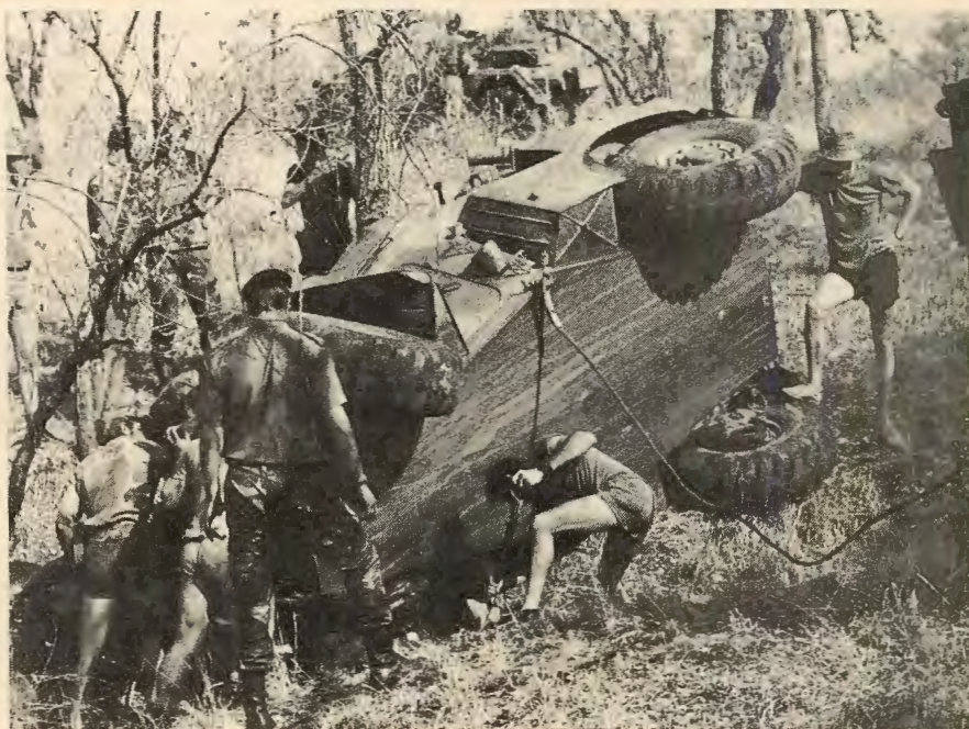
Troopies prepare to right Eland 90 with Mercedes-Benz two-five. (Eland is South African-manufactured copy of the French Panhard AML.)
