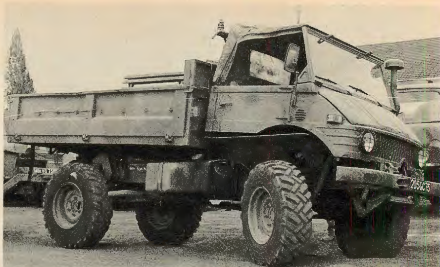
Mercedes-Benz two-five is popular patrol vehicle and troop carrier. Two-five is often mounted with twin 7.62mm Browning MGs.
