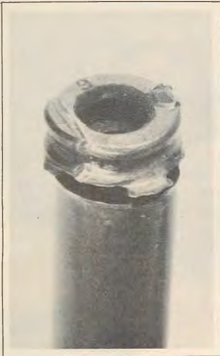
Cause of blowup of 5.56mm cartridge is apparent from obvious, crude removal of military crimp, apparently by woodscrew countersink. See text for details.
