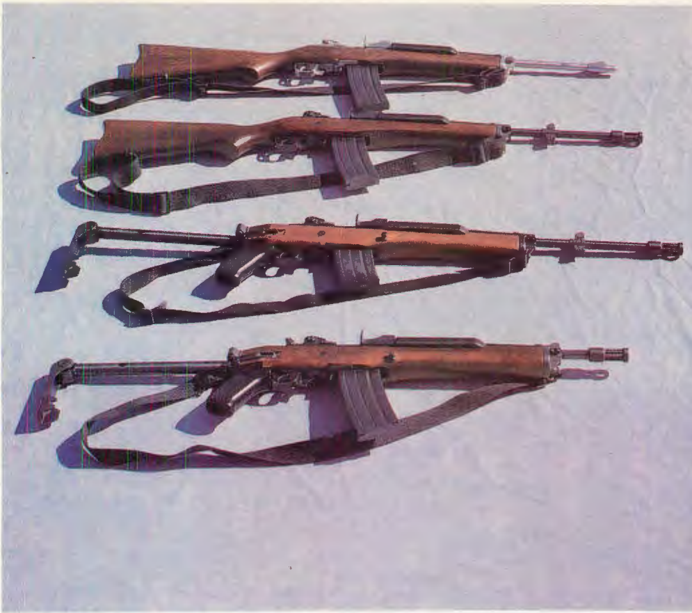
LEFT: Ruger lineup (top to bottom): stainless-steel Mini-14, AC-556, AC-556 with blued-steel folding stock and AC-556K. BOTTOM: Brent Christensen examines receiver of AC-556K and prepares to push release button permitting folding stock to close.
