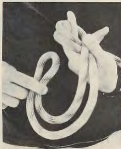
Figure-Eight Knot. Step 2: Form a double loop as if tying an overhand knot.
