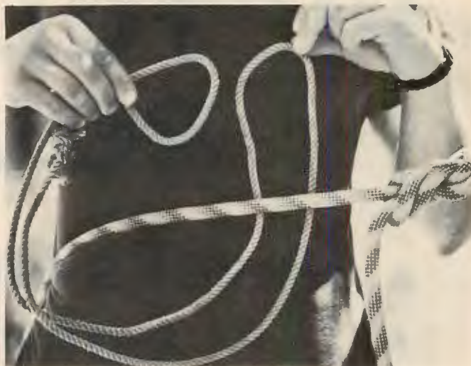
Prusik-Knot System. Step 1: Six or eight feet of 1/4-inch nylon rope forms closed loop when ends are secured with water knot.
