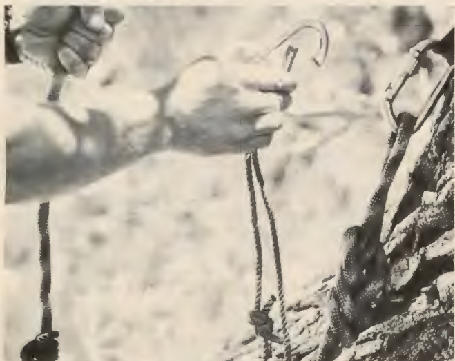
Prusik-Knot System. Step 4: Link prusik system to sling (around trunk) with carabiner. Note: Climbing rope's slack is removed by pulling it with prusik system.
