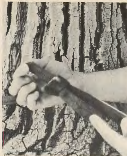
Water Knot. Step 2: Other end of the webbing retraces the overhand knot from opposite direction.
