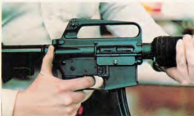
Holding action closed in single fire further muffles sound.
