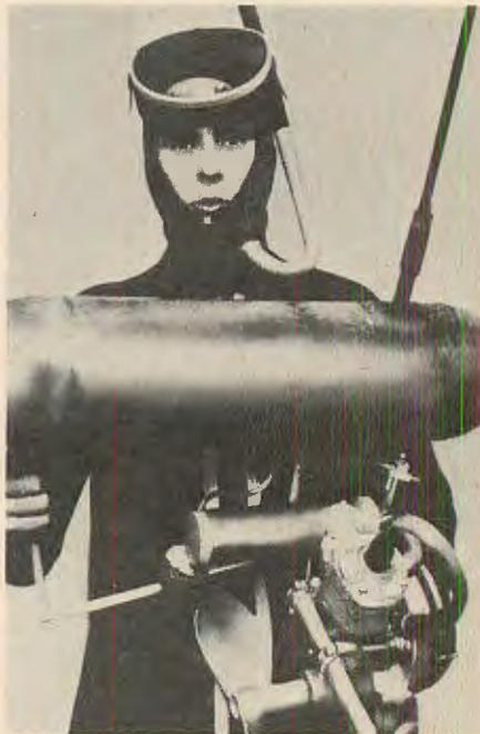
Bernd Boettger holds prototype AquaScooter that carried him across North Sea in 1968. Machine has two-chambered fiberglass tanks, engine, propeller and snorkel-equipped breathing unit, supplying air to both diver and engine.
