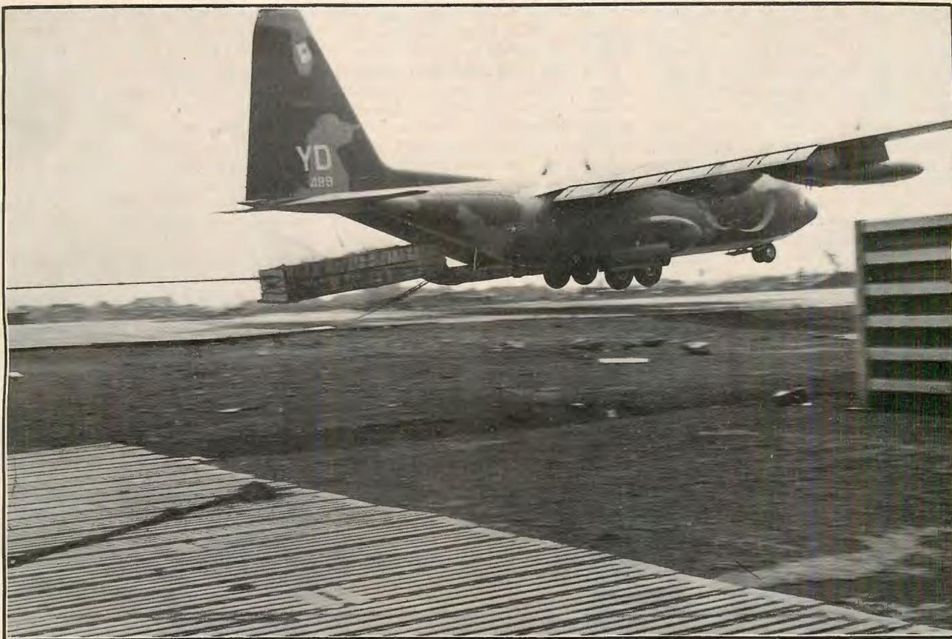
The trailing hook of C-130 Hercules cargo load catches on arresting cable that stretches across Khe Sanh runway. System decreases aircraft's exposure time to hostile fire. Photo: USAF
