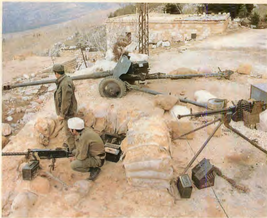
In addition to American-made arms, Israelis supply Christians with many Soviet weapons captured from Arab armies in past actions. From left to right, American .50 caliber Browning AN-M3 aircraft MG, modified for ground use, Soviet 85mm D48 anti-tank/field gun, Soviet 12.7mm M-1939 DSHK.
