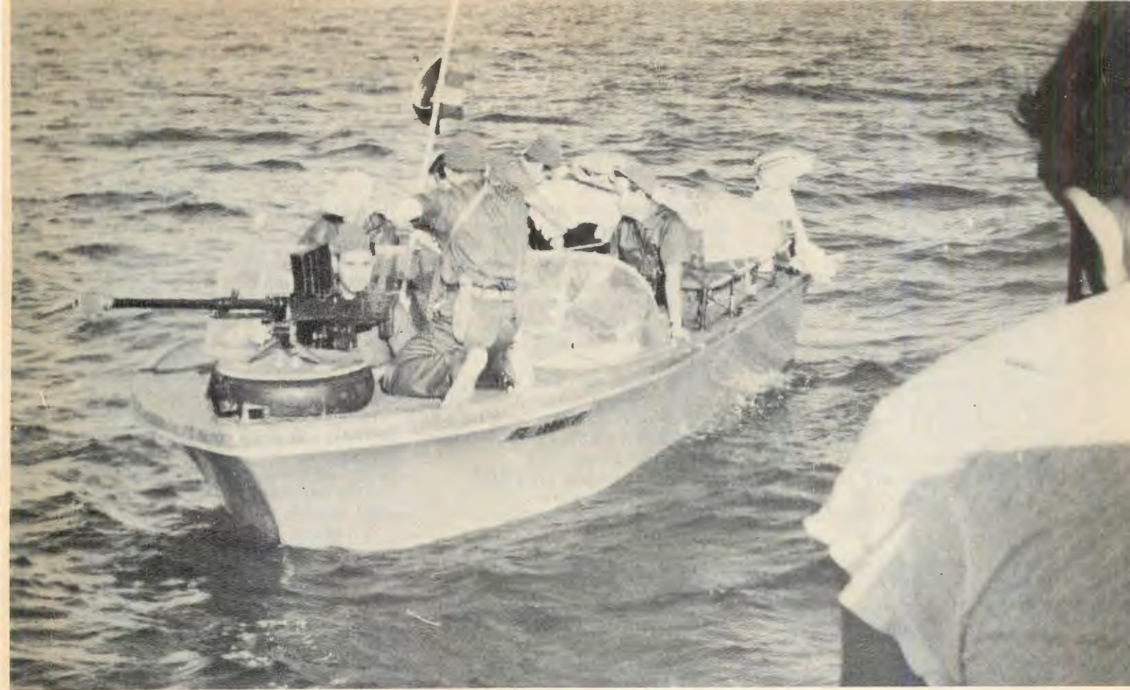
'Commandos L' in March 1963, prior to mission in which they sank Soviet freighter BAKU in Cuban port. WWII semi-auto antitank gun on bow was secured to plywood disk, which was bolted through tire to deck. Tire absorbed heavy recoil of weapon.
