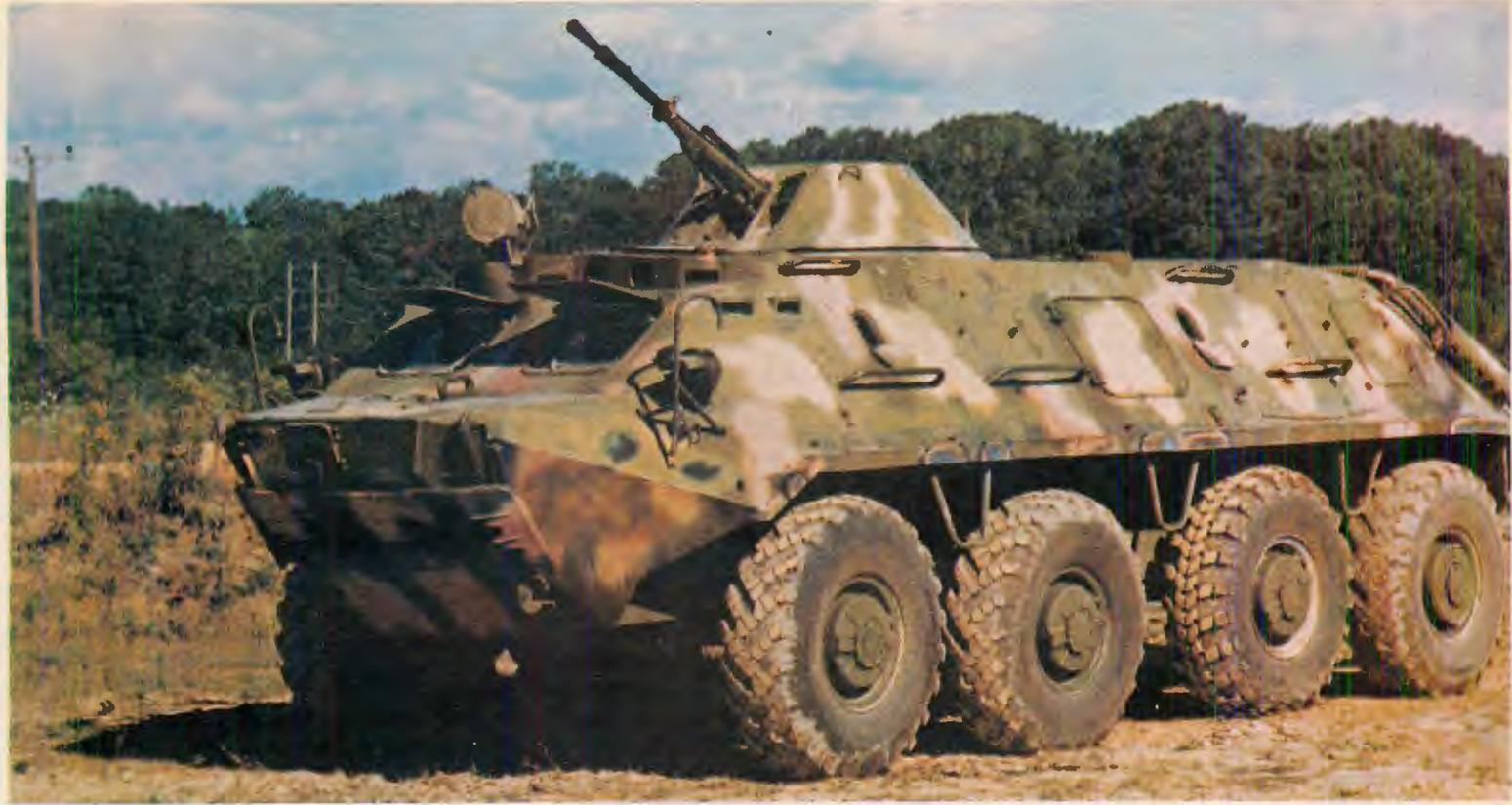
Above: BTR 60 showing 14.5mm main gun; shield just below bow of vehicle is raised when going through water to prevent splash. Photo credit: U.S. Army.
