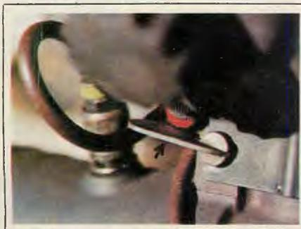
IR devices, since they have own light source, must have ability to focus IR light source with electronic telescope. On this IR unit, is accomplished via small lever mounted below IR lamp assembly.
