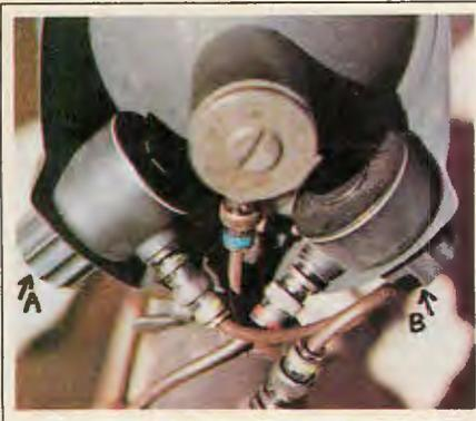
U.S. M3 infrared sniperscope from rear. Knob on left (A) controls electronic focusing of telescope while knob on right (B) allows varying intensity of reticle; consists of small vertical bar of light that appears in field of view. Can be turned off for surveillance and, via rheostat, made progressively brighter for actual sniping work. Center cable (with blue connector) provides power to operate 30-watt IR light source.
