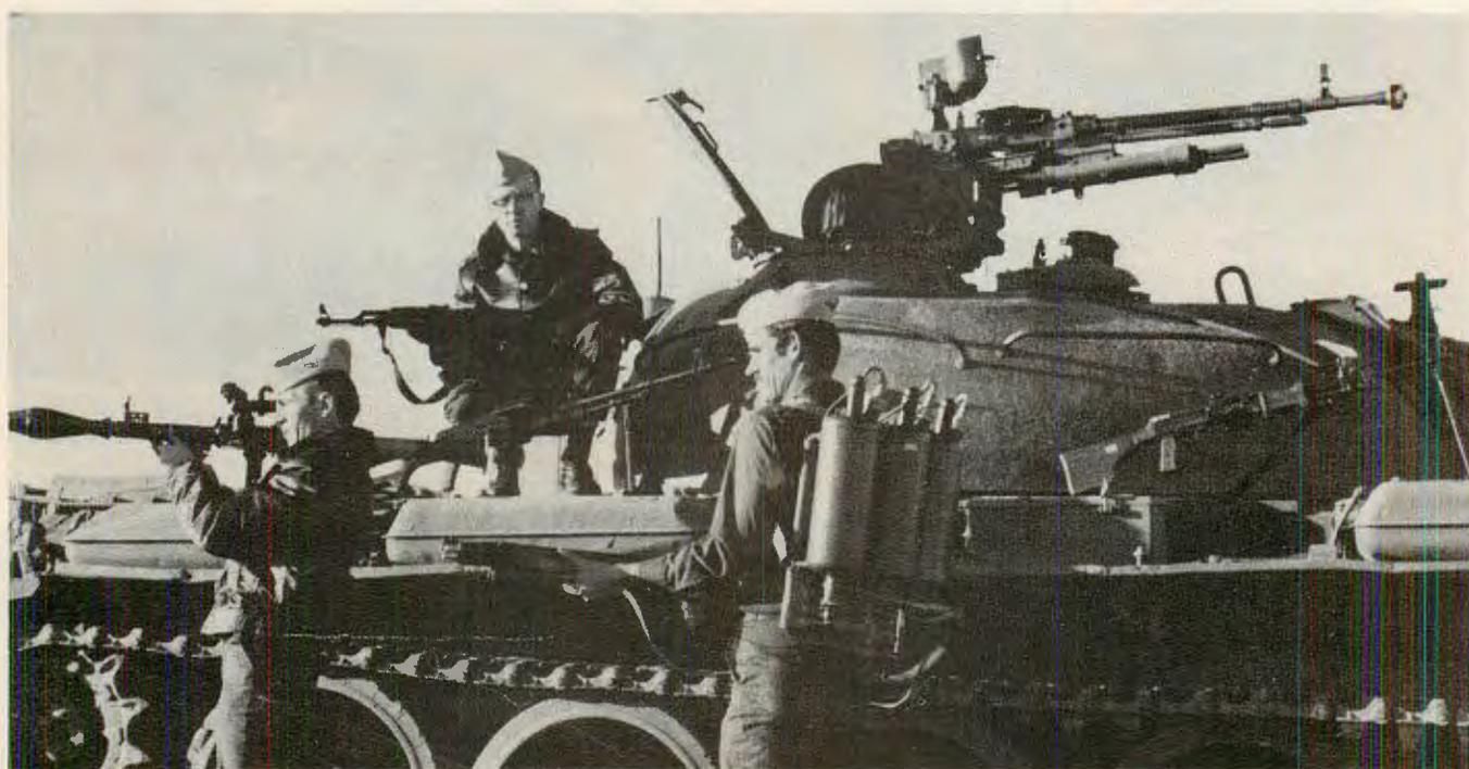
The T-54, 55, and 62 all have four-man crews. The T-54 and 55 mount a 100mm rifled main gun, 7.62 MG, and a 12.7mm (.50 caliber) DShK 1938/46 heavy MG for anti-aircraft use. Some of these tanks have chemical, biological, radioactive (CBR) equipment, which may be manually operated or activated by an atomic weapon flash.
