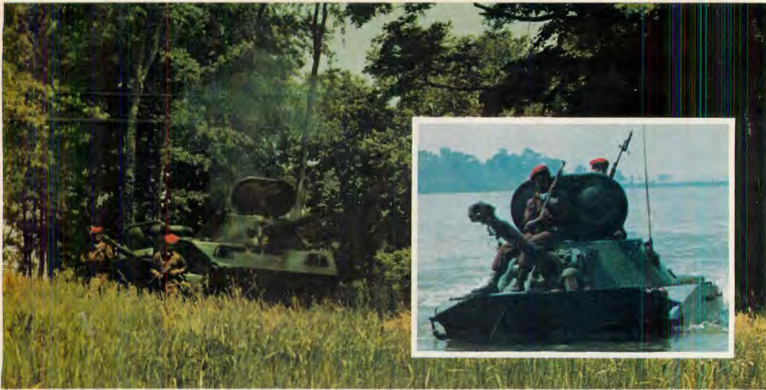
Above: Ft. Hood's OPFOR troops take to field accompanied by PT-76 light, amphibious tanks. Note distinctive uniforms. Photo credit: U.S. Army. Inset: One of Ft. Hood's PT-76 amphibious tanks (14.6 tons, 76.2mm gun,
