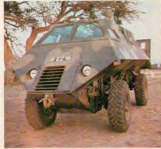
Above: Front view of Bullet, prototype armored infantry fighting vehicle, built by Rhodesian Armored Corps. After 10,000-kilometer road test, Bullet will be blown up by captured Russian landmine to determine its resistance to blast and heat.
