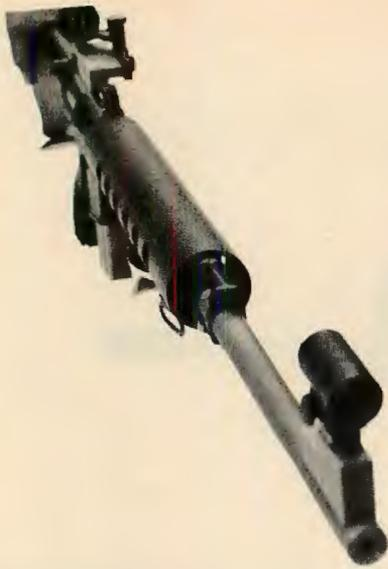
Note front sight blocks and no-contact, free-floating barrel.
