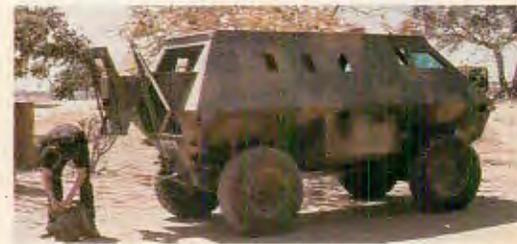
Above: Side view of Bullet. Note firing ports. Carries crew of 10. Vehicle commander leads squad when they dismount. Production version will mount .30 or .50 cal MGs or 20mm cannon.
