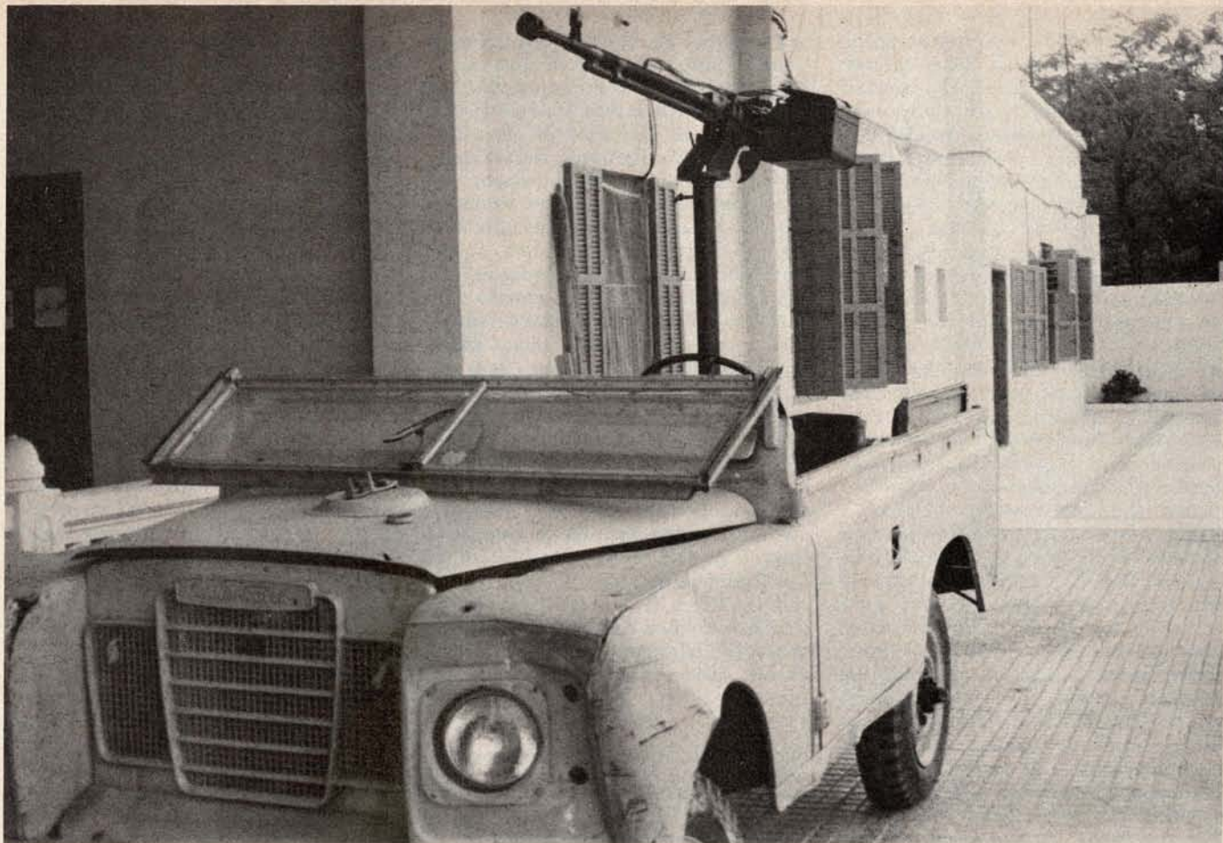
This slightly dinged Land Rover belongs to Falangist forces and carries 12.7mm Daska HMG. Light trucks and similar vehicles mounting medium or heavy machine guns are common to all factions.
