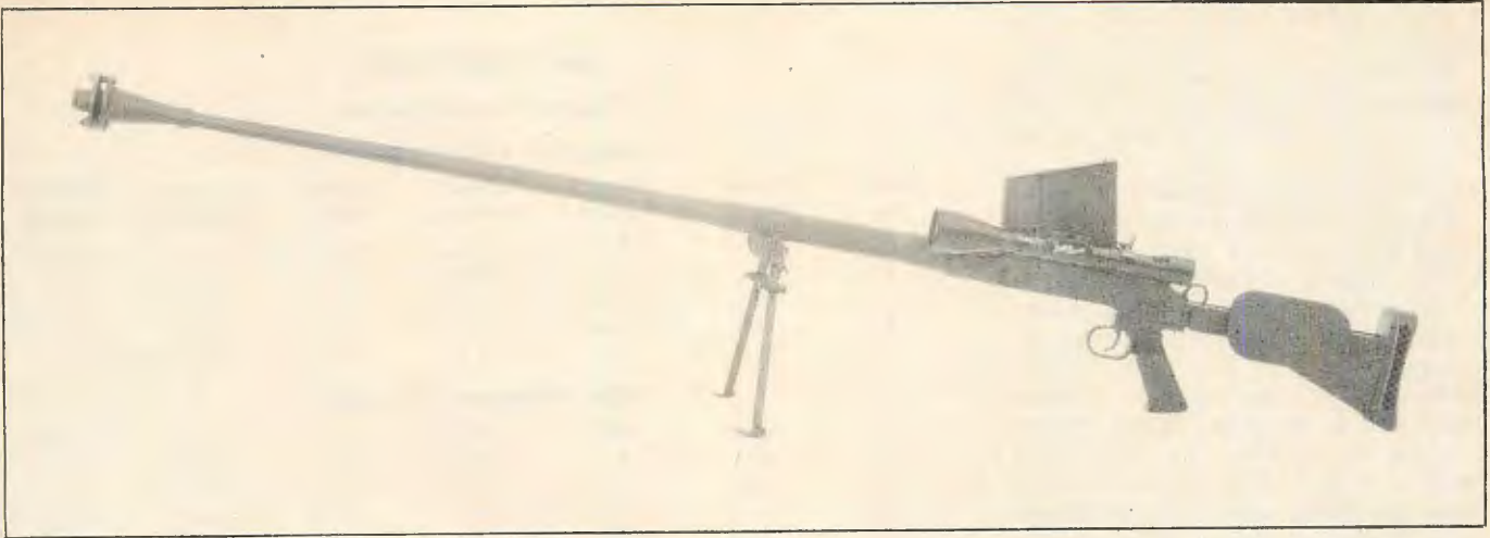
.50 caliber Flechette Rifle developed in 1969 for use against enemy personnel in Southeast Asia. Boys AT-rifle action, smoothbore barrel, Weatherby telescope formed nucleus of this unique weapon. (Photo credit: Donald Stoehr.)
