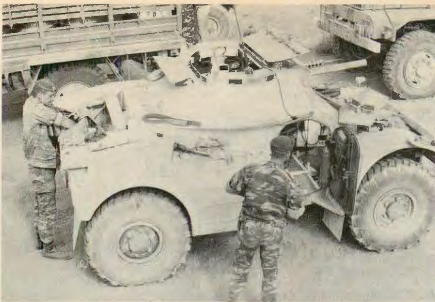
Grand Barre. Legionnaire digs through kit on back of AML60, light armored car carrying 60mm mortar.
