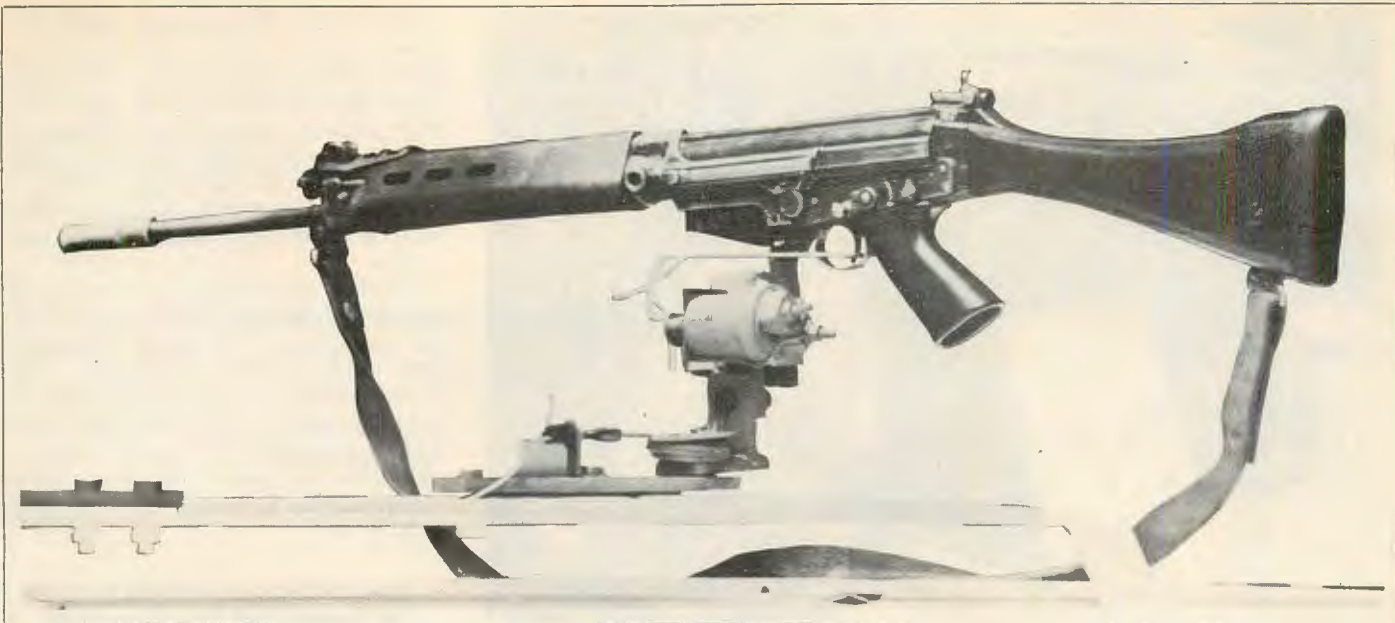
Rooftop Ambush Remote Firing System with FN/FAL mounted in place. The effectiveness of this weapon system is limited, in part, by 20-rd. magazine capacity of the FN.
