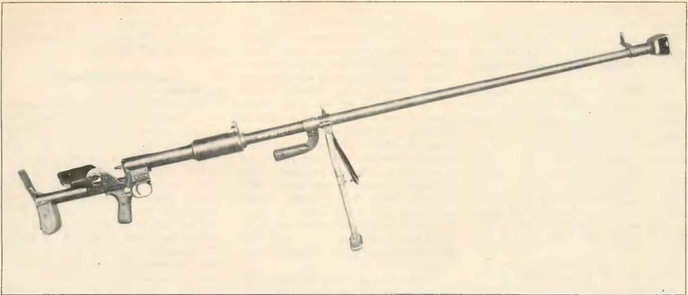
Soviet PTRD1941 14.5mm anti-tank rifle, employed by Communist forces during Korean conflict, served as basis for Capt. Brophy's special .50 cal. sniping weapon. (Photo credit: U.S. Army.)
