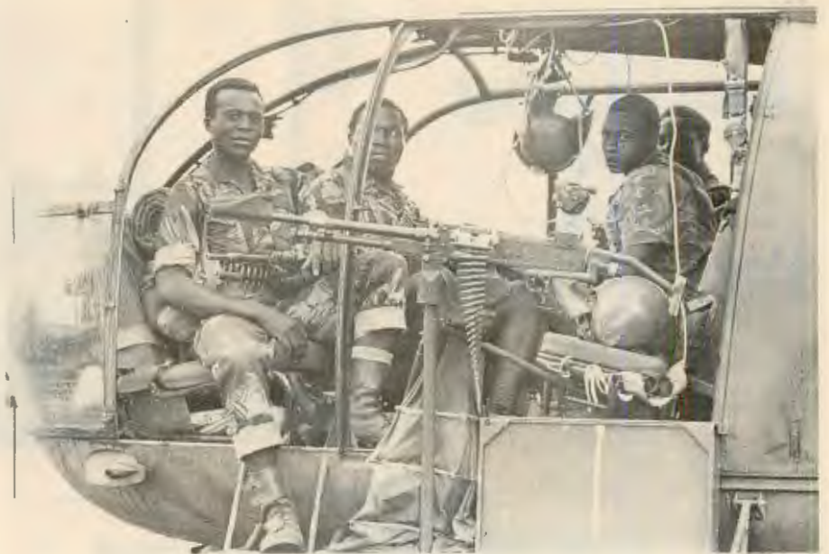
Rhodesian reaction "stick" on call. Note improvised butt stock on MAG LMG.
