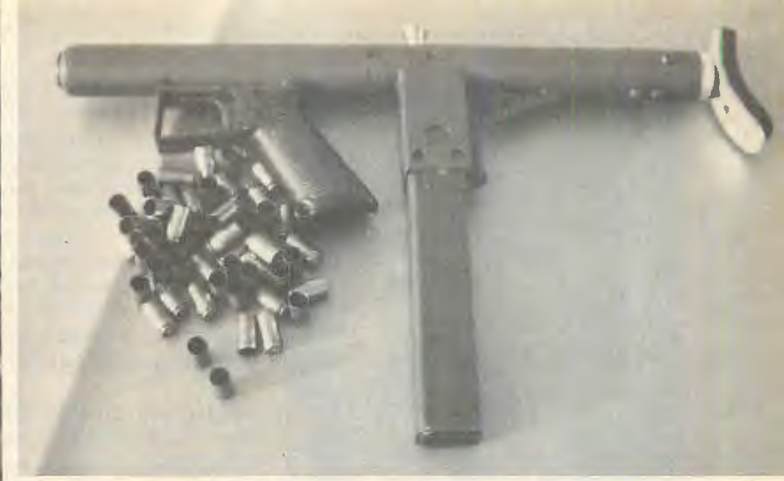
Sidewinder is only SMG to fire pistol cartridge. Magazine to rear of pistol grip enhances balance.
