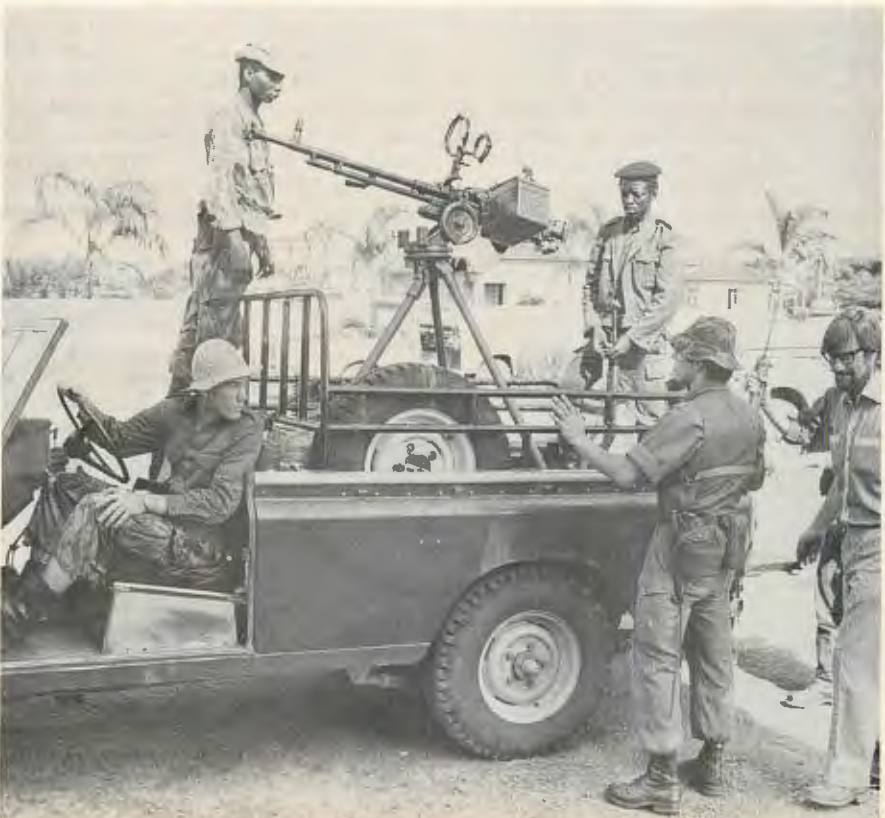
Below: Mercs will continue to play significant roles in African conflicts as majority of black troops are poorly trained, disciplined; have little technical expertise. Note DShK 38/46 12.7mm heavy machine gun mounted in Land Rover with anti-aircraft sights.
