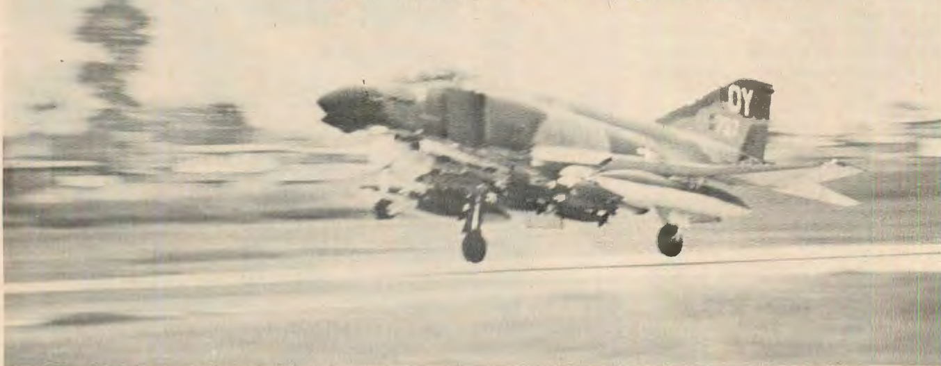
F-4D taking off from UDorn during Linebacker operation. It carries 12 Mk-82 500-lb. bombs, one ECM pod and three AIM-7 Sparrow air-to-air missiles. The outside stations are holding jettisonable fuel tanks.
