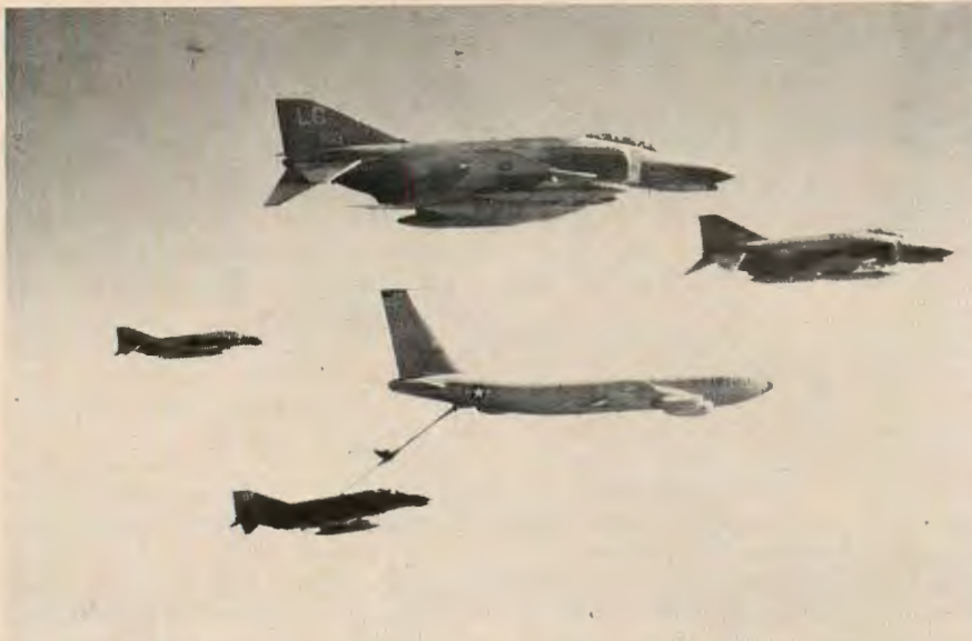
F-4's refueling with a KC-135 tanker enroute to a Migcap mission over Hanoi. The two F-4s in the foreground are E models with 20mm Vulcan cannon in the nose; two in background are D models.
