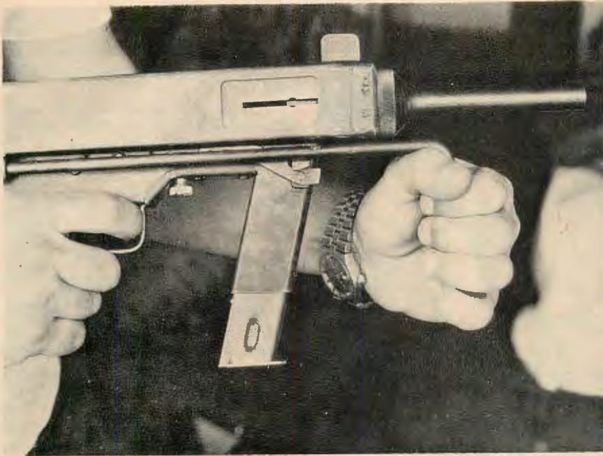
Prototype R-76 appears crude and ugly but is easy to manufacture. Note reversed wire stock that can serve as fore-grip.
