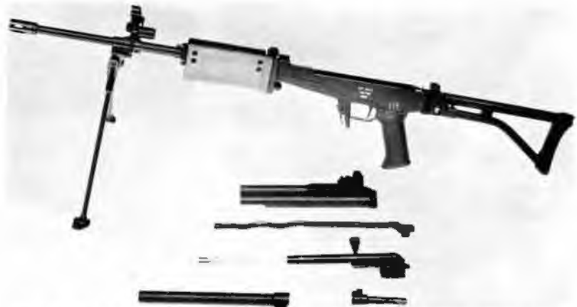
Here the Galil is shown field-stripped for cleaning and maintenance. In this photo, anyone who is remotely familiar with the AK47 will immediately notice that the parts, for all practical purposes, are identical.
