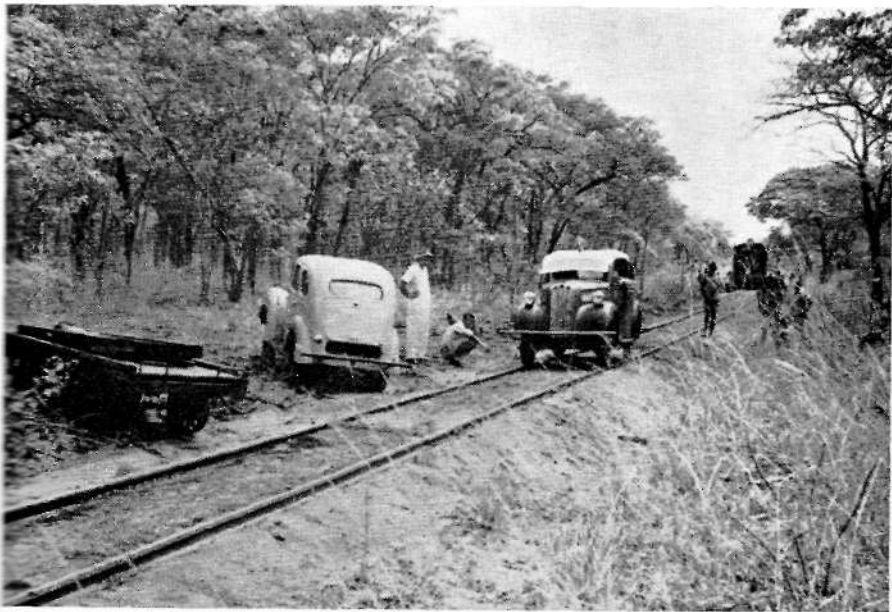
Motor trolleys crossing near mile 41 in October, 1963. The trolley and trailer lifted clear of the track would be replaced on the track when the train in the distance had passed.
